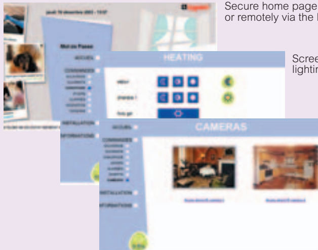
Cameras are used to view the inside of the home at the user's request or automatically when an alarm is triggered (intrusion or detection)
